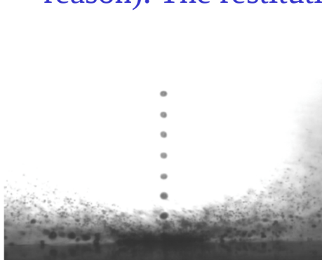
Experiment, normal impact with K = 4591
